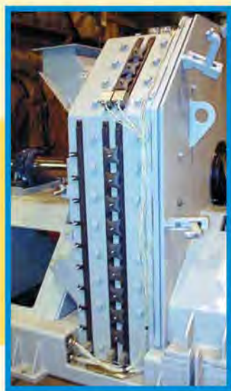
Heaters (shown with guards removed) are installed on the "H" Mill housing to retard build-up of wet material.
