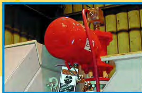
Air Cannons are mounted at the intake and discharge to help prevent build up of wet material.
